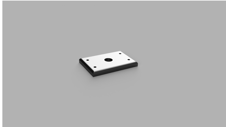
Figure 6: Sketch with estimated measurements for the triple clamp, showing M8 screw holes and a center thread about 1" in diameter
